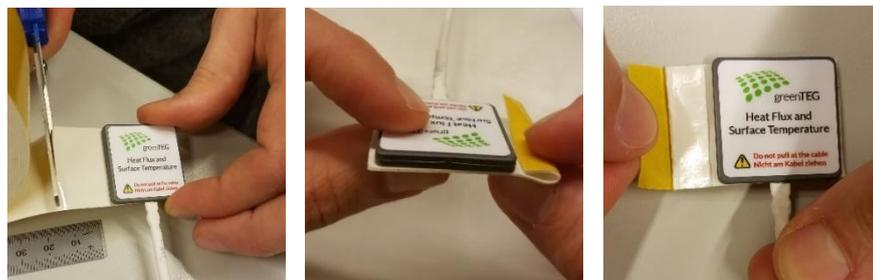
Figure 3 How to mount the sensor correctly
