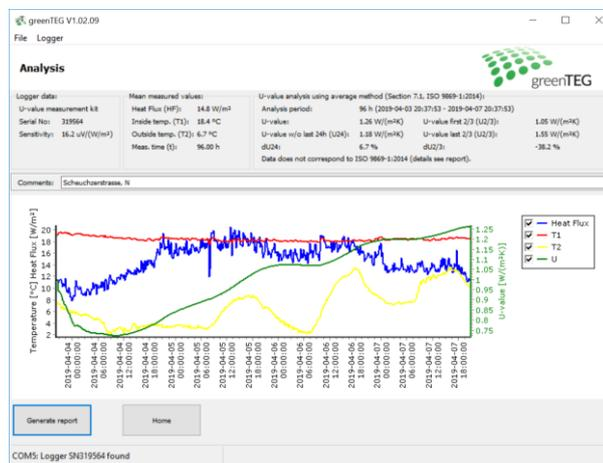
Figure 4: Analysis window showing U-value output and sensor data graphs.
