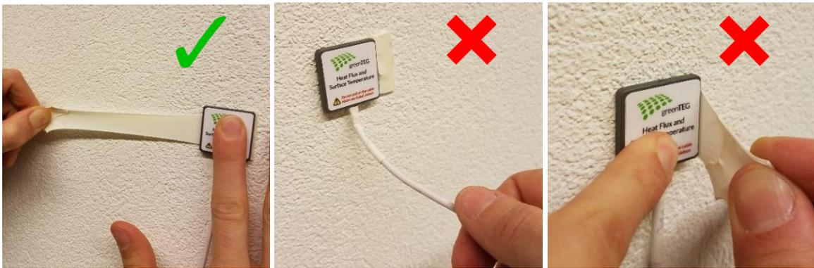
Figure 6 How to demount the sensor correctly
